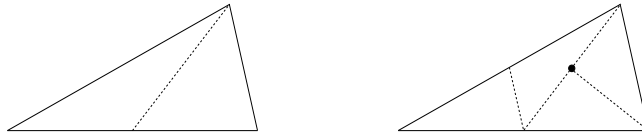
Figure 1: The classical longest-edge bisection algorithm may produce triangulations that are not face-to-face. Broken lines stand for new bisections.
