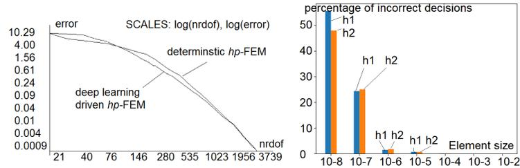
**Fig. 3.** **Let panel:** The comparison of deterministic and DNN  $hp$ -FEM on original L-shape domain. **Right panel:** The sizes (horizontal  $h_1$  / vertical  $h_2$  directions) from  $10^{-2}$  (right) down to  $10^{-8}$  (left) of the elements where MPL network made incorrect decisions during verification.
