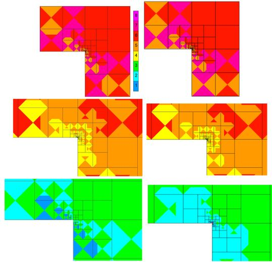
**Fig. 2.** The mesh provided by the deterministic  $hp$ -FEM algorithm and by the deep learning-driven  $hp$ -FEM algorithm. Different colors denote different polynomial orders of approximation on element edges and interiors. The original L-shape domain. Zoom 1x, 1000x, 100000x towards the center. The sequence of  $hp$  refined meshes generated by deterministic algorithm (left panel) and DNN driven algorithm (right panel).
