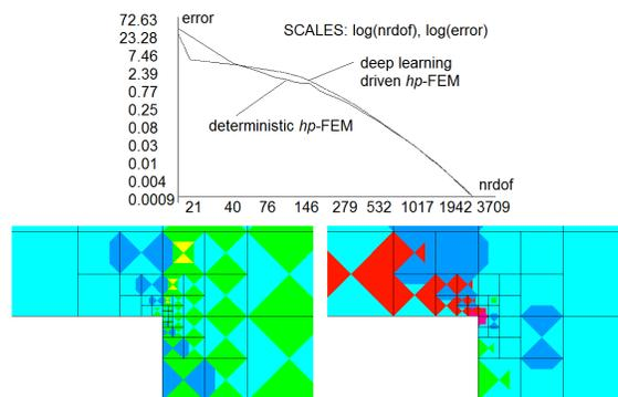
**Fig. 5.** The convergence for deterministic and DNN hp-FEM algorithms for the L-shape with b.c. rotated by 45 deg. The meshes of the deterministic *hp*-FEM algorithm and by DNN driven *hp*-FEM algorithm for the L-shape domain with b.c. rotated by 45 deg. Zoom  $10^5$ x times.
