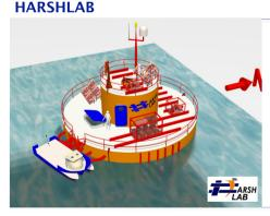
HarshLab is a floating platform that serves as an offshore laboratory in real marine environment. It will be installed at BiMEP facilities in the Basque coast. Its functionality consists of:
